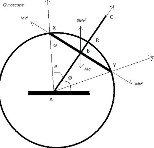
The higher the rotational rate  $\omega$ , the less the relative effect of gravity and the more stable in orientation the gyroscope shaft will remain. Without a support point, there will be no spherical effect and the gyroscope will have only the planar energies acting outward equally around the disc, keeping it in the same shaft orientation until disturbed.
